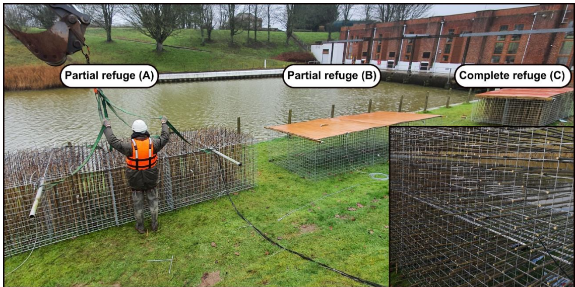
Figure 5.3 Photographs of the three artificial habitats installed upstream of Tydd PS (52.738804N, 0.162728W). From left to right, partial refuge (A), partial refuge (B) and complete refuge (C). Inset photo shows bamboo canes installed through apertures in steel cages. Positions of artificial habitats differ in this photo from the final installed positions (Figure 5.1c).
