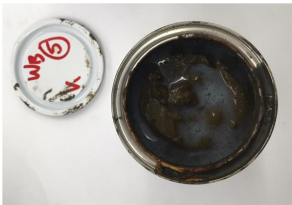
Figure 7.16: Instability in emulsion formulation after just 24 hours.
