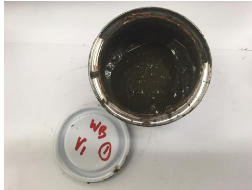
Figure 7.14: Emulsion water-based ink formulation made on HMI mini attritor.
