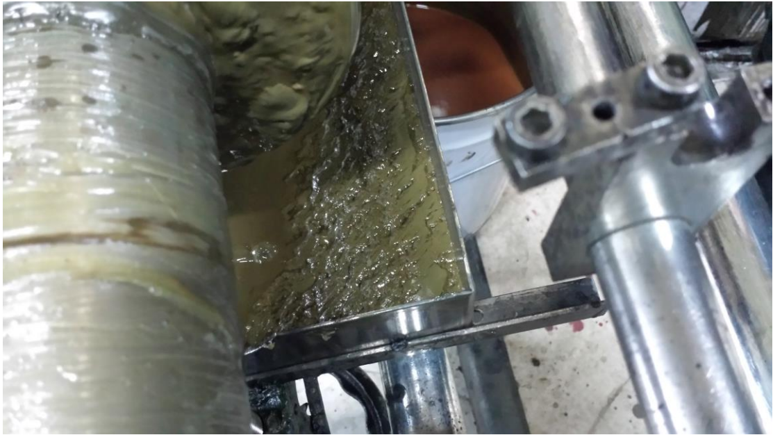
Figure 7.3: Gelling of HL0103 inside the printing machine
