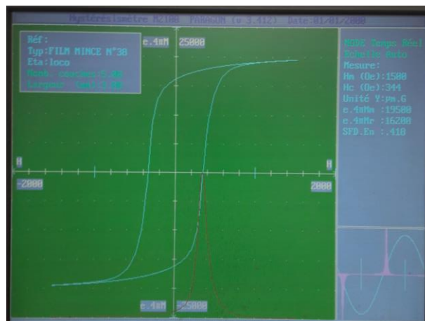
Figure 7.19: BH loop results of the mini attritor condensation formulation.
