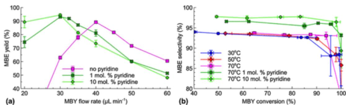
Fig. 9 (a) MBE yield as a function of liquid flow rate in MBY hydrogenation in the presence of pyridine over a Pd–Bi/TiO<sub>2</sub>-coated capillary reactor at a 10 mL/min hydrogen flow rate, and (b) MBY conversion vs. MBE selectivity plot for the studied reaction conditions.
