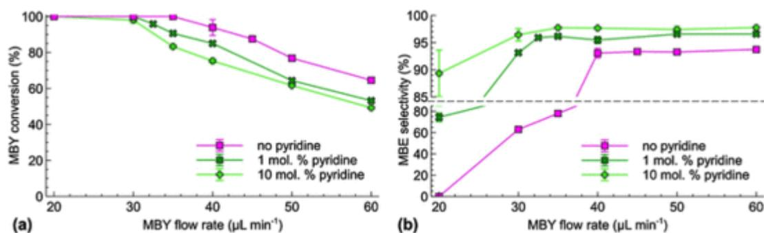
Fig. 8 (a) MBY conversion and (b) MBE selectivity as a function of liquid flow rate in MBY hydrogenation in the presence of pyridine in a Pd–Bi/TiO<sub>2</sub>-coated capillary reactor at a 10 mL/min hydrogen flow rate.
