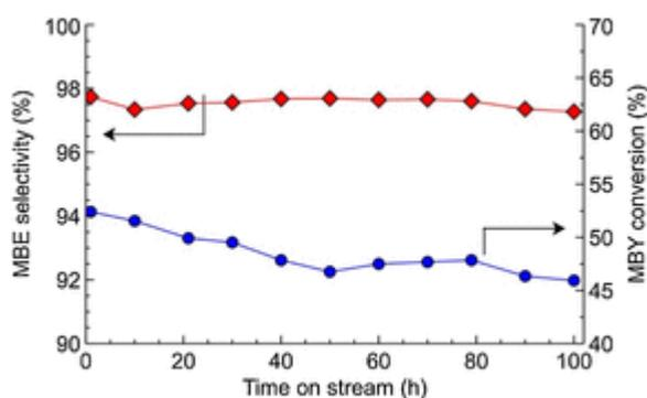
Fig. 11 MBY conversion and MBE selectivity over a Pd–Bi/TiO<sub>2</sub> coating in a 2 m capillary (0.53 mm i.d.) in the presence of 1 vol.% acetic acid. Liquid flow rate of 20  $\mu\text{L min}^{-1}$  and hydrogen flow of 5 mL  $\text{min}^{-1}$  (STP), 50 °C, ambient pressure, 0.2 bar pressure drop.
