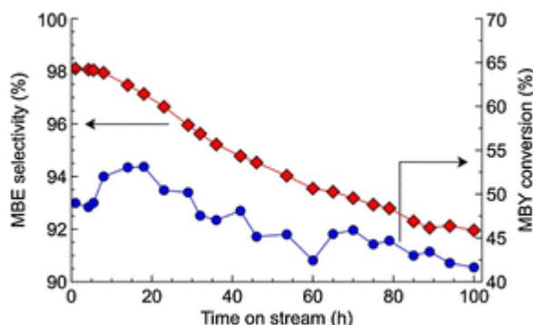
Fig. 10 MBY conversion and MBE selectivity over a Pd–Bi/TiO<sub>2</sub> coating in a 2 m capillary (0.53 mm i.d.) in solvent-free MBY hydrogenation. Pd loading in the coating is 3.4 wt.%, Pd/Bi molar ratio is 7. MBY flow rate is 20  $\mu\text{L min}^{-1}$ , hydrogen flow rate is 5  $\text{mL min}^{-1}$  (STP), temperature is 50  $^{\circ}\text{C}$ , ambient pressure, 0.2 bar pressure drop.
