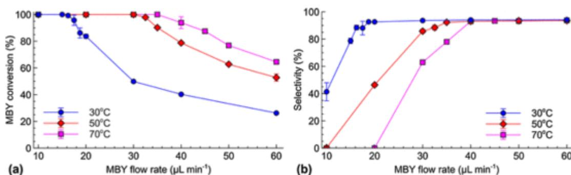
Fig. 6 (a) MBY conversion and (b) MBE selectivity as a function of MBY flow rate in solvent-free MBY hydrogenation in a Pd–Bi/TiO<sub>2</sub>-coated capillary reactor at a hydrogen flow of 10 mL min<sup>-1</sup> and different reaction temperatures.
