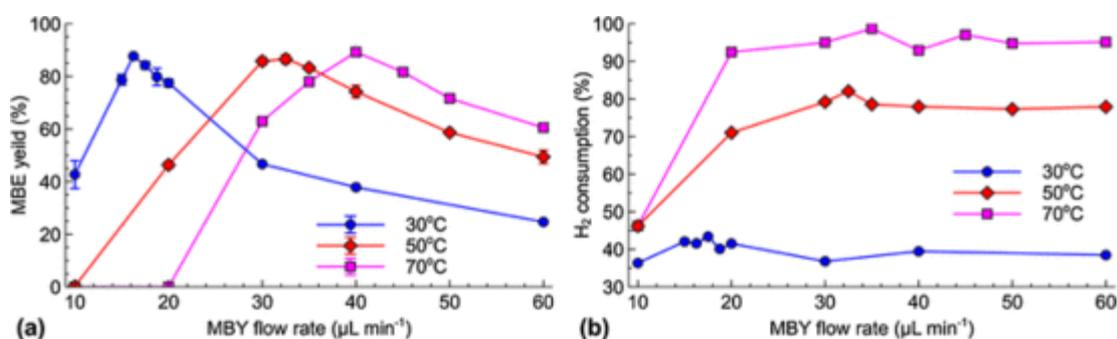
Fig. 7 (a) MBE yield and (b) hydrogen consumption as a function of MBY flow rate in solvent-free MBY hydrogenation in a Pd–Bi/TiO<sub>2</sub>-coated capillary reactor at a hydrogen flow of 10 mL min $^{-1}$  and different reaction temperatures.
