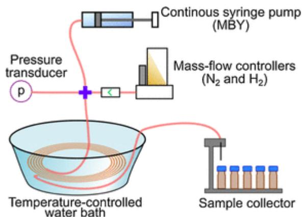
Fig. 2 Scheme of the hydrogenation capillary reactor Schematic view of the capillary reactor.
