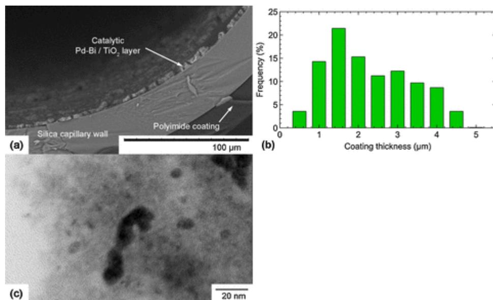
Fig. 4 (a) SEM image of the Pd–Bi/TiO<sub>2</sub> wall-coated capillary, (b) axial coating thickness distribution obtained from 25 cross-sectional SEM images, and (c) TEM image of the Pd–Bi nanoparticles.
