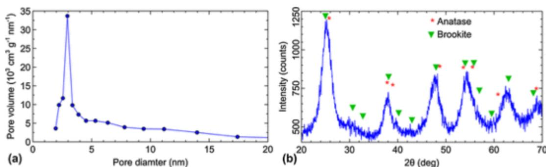
Fig. 3 (a) Pore size distribution and (b) PXRD pattern of Pd–Bi/TiO<sub>2</sub> coating obtained in a 1.6 mm glass tube.
