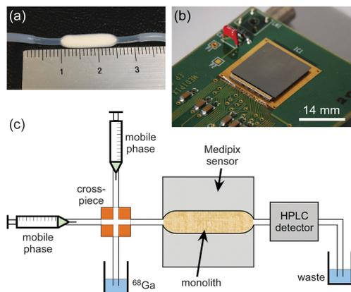
**Fig. 1** (a) Silica-based monolithic column encased in heat-shrink tubing. (b) Medipix positron detector, featuring a  $14 \times 14 \text{ mm}^2$  sensor area. (c) Schematic of the experimental setup, with the monolith placed above the Medipix sensor, and featuring a cross-injection system and a standard sodium iodide radio-HPLC detector.
