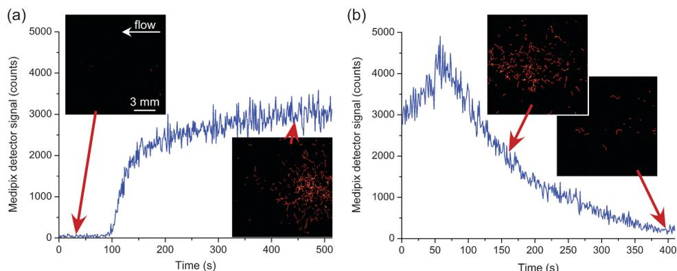
**Fig. 4** Trap and release of  $^{68}\text{Ga}^{3+}$  on the silica-based monolith, with the positron detector showing the activity in real-time. (a) Trapping in phosphate solution (0.4 M). (b) Release in citric acid (0.1 M). The flow of solution was right-to-left in the images.
