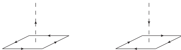
Figure 13. Using a right-handed convention a plaquette has a natural orientation vector associated with it.
