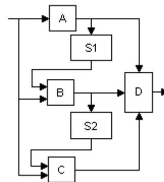
Fig. 4. Dynamic system with two backup components.
