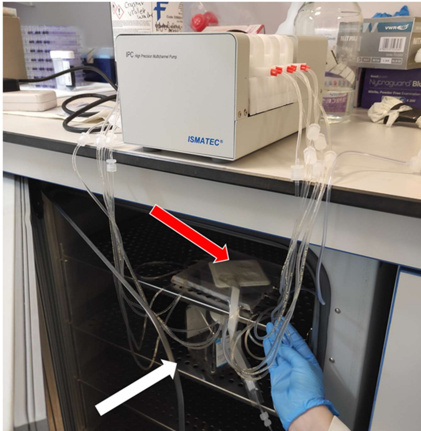
Figure 5. 15 Setup of bioreactor system for negative pressure application on scaffolds inside a cell culture incubator at 37° C and 5% CO 2 .
