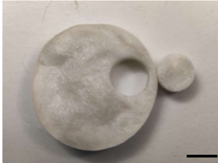
Figure 5. 1 Example of collagen sample punched out of a 35 mm porous scaffold. Scale bar = 10 mm.
