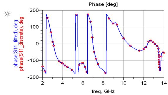
Fig. 3. The calculated  $S_{11}$  phase
