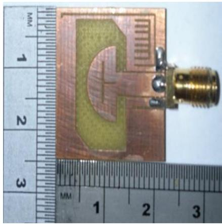
Fig.5. Dimensions of antenna.
