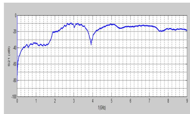
Fig. 9.  $S_{21}$  as a function of frequency for broadside antennas,  $d=100$ mm.
