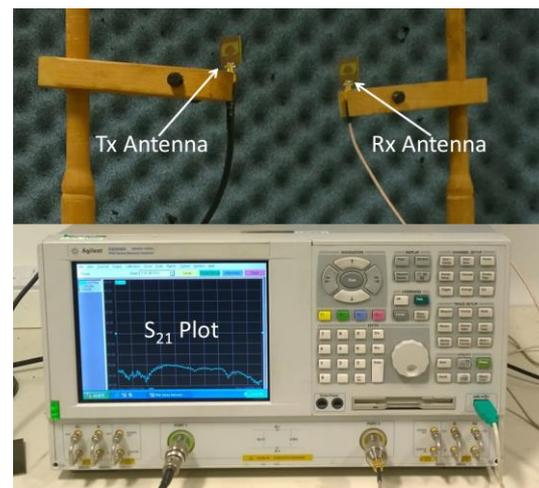
Fig. 8. Arrangement of antennas (Top) and Measurement system (bottom).
