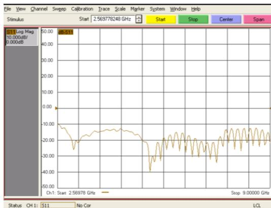
Fig.6. Return loss  $S_{11}$  measured by VNA.
