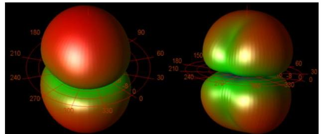
Fig.4. Radiation for 6.80 GHz (left) and 9.40 GHz (right).
