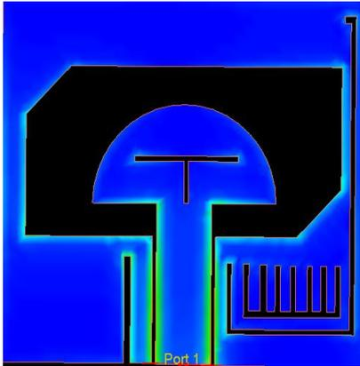
Fig. 1. Layout of Slot loaded CPW-FED Antenna and Current distribution for the frequency 6.80 GHz.
