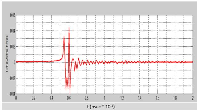
Fig. 10. Time domain analysis of the frequency domain measurements, 0 – 20 ns scale.
