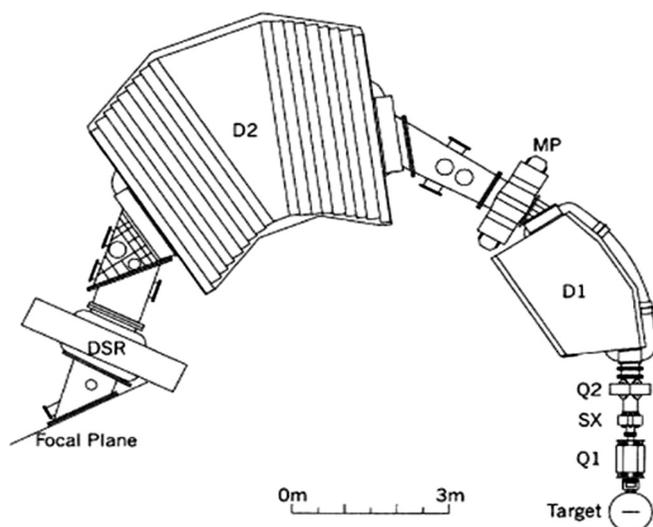
FIG. 1. Schematic layout of the Grand Raiden Spectrometer at RCNP. The dipole magnet for spin rotation (DSR) was not used in the present experiments, but it is a part of the permanent installation. Figure from Ref. [69].
