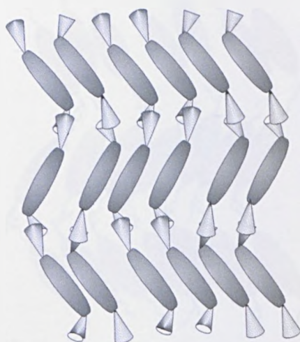
Figure 36(b):- Bent “zig-zag” structure of the SmC_A^* phase (the “cones” represent the rotational distributions of the terminal branched and unbranched chains)
