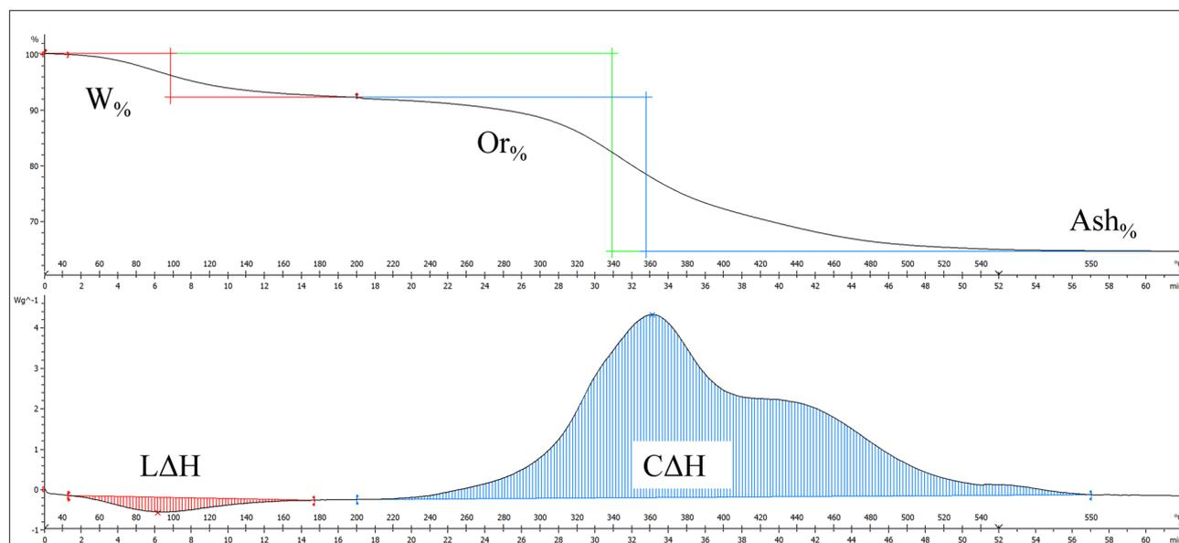
**Figure 3.** Graphic representation of thermal analysis experiment. Example of thermogravimetric (A) and differential scanning calorimetry (B) curves. The first weight loss represents the bone matrix dehydration and matches with the endothermic peak responsible for triple helix thermal denaturation (LAH and W%). The second weight loss (Or%) represents organic combustion (CAH) and matches the DSC curve. Subtracting the entire weight loss (Ash%) from 100, it is possible to obtain mineral content.
