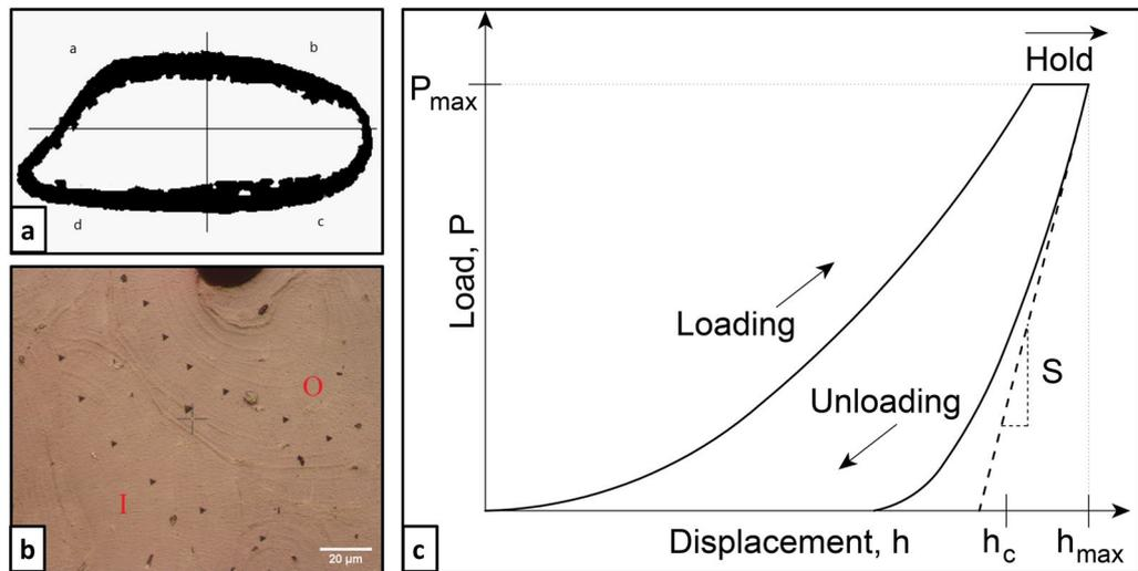
**Figure 2.** Steps for nanoindentation. The four quadrants used to divide the cortical area for sampling in order to perform porosity calculation (A) and nanoindentation impressions (B) on the osteon (O) and the surrounding interstitial bone (I) divided by the cement line (red dashed line). (C) Shows the typical load/indentation depth curve used to acquire mechanical parameters.
