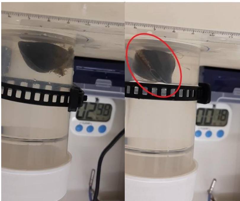
Fig. 5.6 and 5.7 Frames from the recorded videos showing the respirometer assays for mussels with closed (left) and open (right) valves (highlighted in red) and the recorded time
