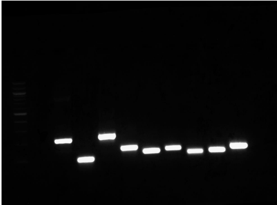
Fig. 4.22 Agarose gel 2% (2%, GelRed, run at 80V) after a qPCR run, showing the final sets chosen. From left to right: 100 bp NeB DNA ladder, sod (208 bp), MeER1 (94 bp), MeER2 (232 bp), Me28S (143 bp), Me18S (116 bp), cat (126 bp), CA2 (102 bp), EF1α (105 bp), hsp70 (127 bp)
