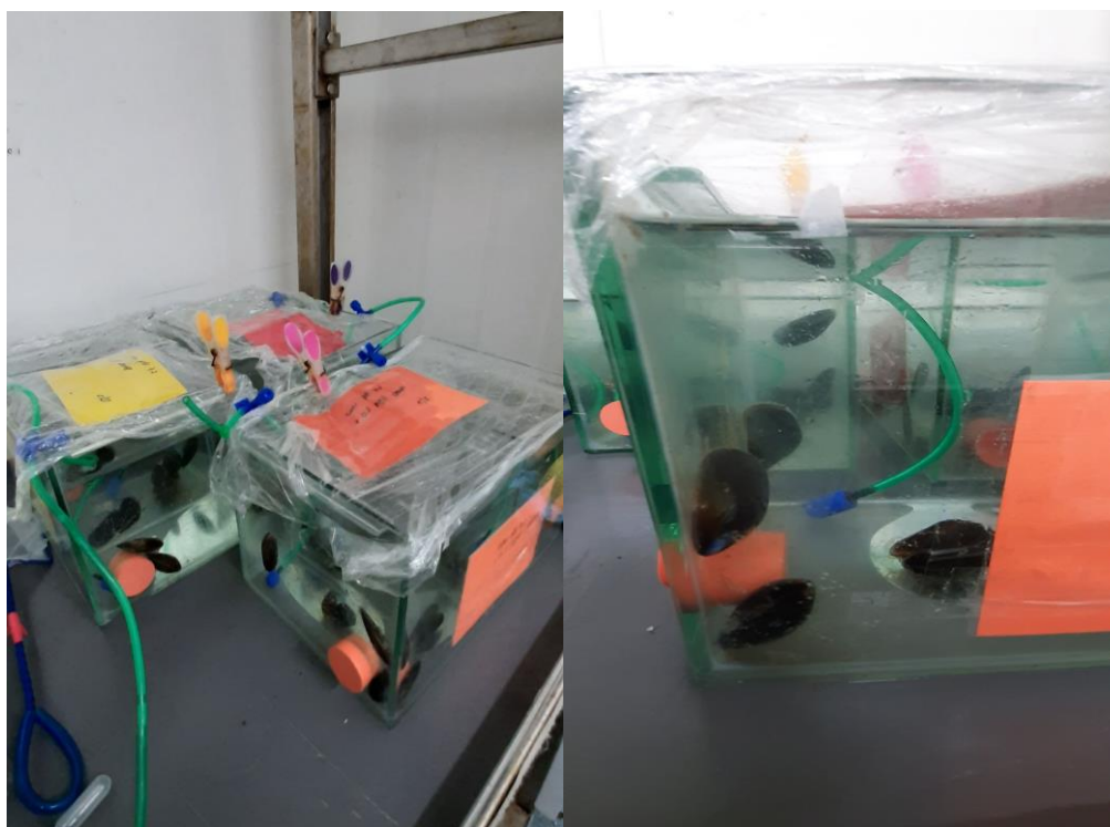
Fig. 4.10 and 4.11 Details of mussels (5 individuals for 4 litres) in the exposure tanks, covered in non-PVC cling film
