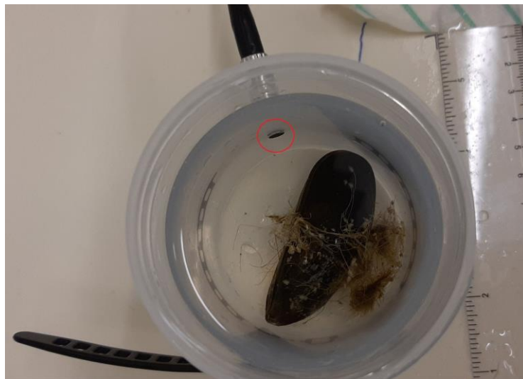
Fig. 5.5 Details of the respirometer assay (before the lid closure) with the sensor spot highlighted by the red circle
