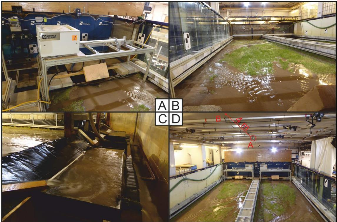
Figure 5.3: Selections of images of the experiments taken during events 11-14 of run 2. A) Close up of inlet and sediment feeder. B) Longitudinal view of bed 2, looking downstream from inlet. C) Downstream weir and water and sediment collection basin(s). D) Upstream view of both beds including cameras positioned 2.5 m above the bed on the ceiling, Faro scanning locations A and B are located directly above the central wall, 2.5 m above the bed and 4 m apart.
