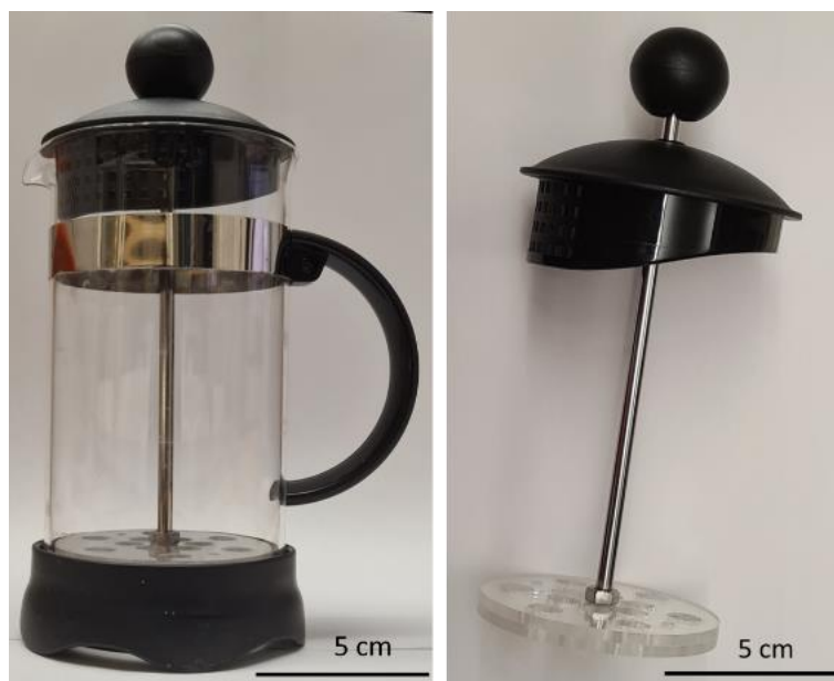
Figure 58 Cafetière setup for Ni 2+ adsorption from water sample with electrospun PCL/chitosan/PEO nanomat.
