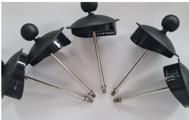
Figure 93 Variation in basket mounting thread in the modified plunger causing different basket mounting strength – shorter thread often led to resin leakage.
