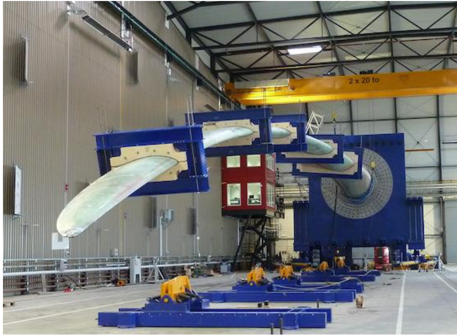
Figure 1.2. Wind turbine blade set up for load testing [26]
