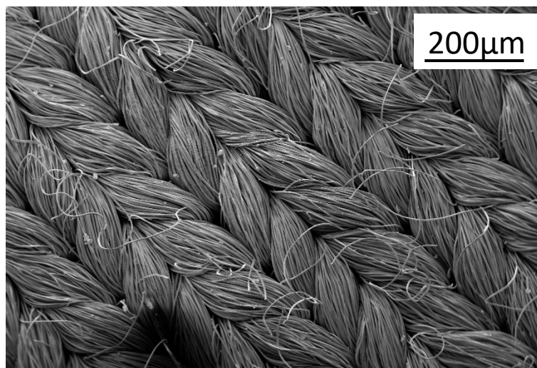
Figure 3.22. Lower magnification image of unreacted polyester/lycra textile waste feedstock
