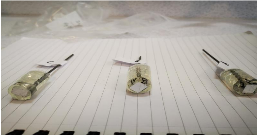
Figure 4. 26: Magnesium alloy specimens namely Mg-10wt%Gd, Mg-10wt%Gd-0.4wt%Zr and Mg-5wt%Gd-5wt%Nd-0.4wt%Zr categories before corrosion test.
