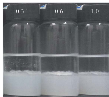
Fig. 8 Photograph of mixtures of n -decane and aqueous phases (1 : 1) containing 0.5 wt% alumina nanoparticles in combination with an equimolar mixture of SDS and DDAA (amidinium/cationic) at different concentrations taken 24 h after homogenisation. Concentration of the individual surfactant in mM is given.
