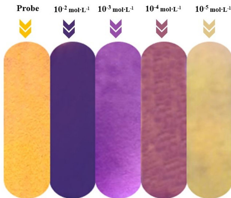
Figure 6. Characterization of fluorescence changes in PCA detection of arginine at different concentrations.
