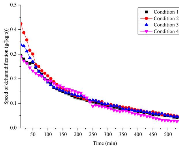
**Figure 11.** Variation of the speed of dehumidification of the solar solid dehumidification/regeneration bed with time.
