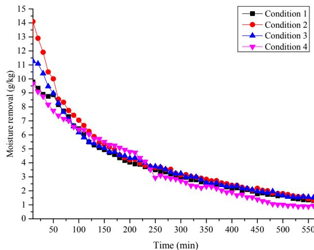
**Figure 9.** Variation of the moisture removal of the solar solid dehumidification/regeneration bed with time.
