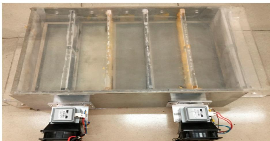
**Figure 4.** Image of the solar solid dehumidification/regeneration bed.
