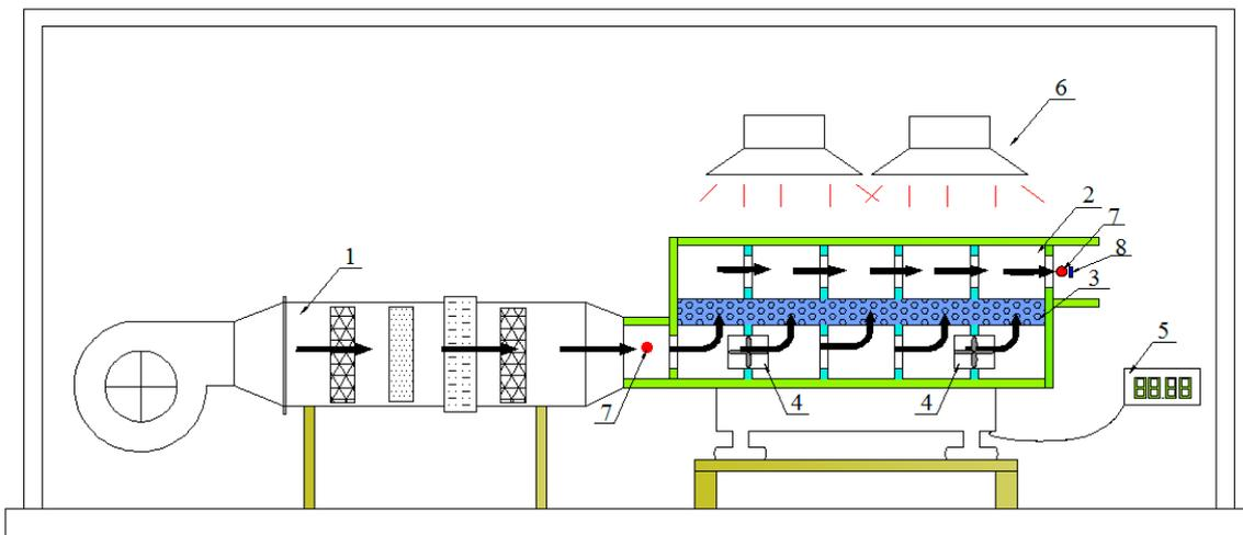
**Figure 2.** The structure of the test rig: 1—DC air conditioner; 2—solar solid dehumidification/regeneration bed; 3—silica gel; 4—microwave generator; 5—electronic scale, 6—xenon lamps, 7—temperature/humidity sensor, 8—Pitot tube anemometer.
