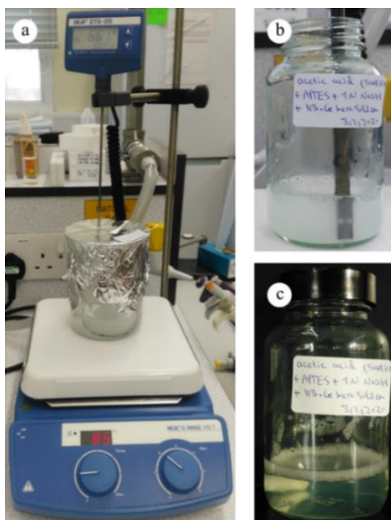
Figure 2.6. (a) The setup used for the synthesis of AS-coated silica, (b) initial turbid dispersion and (c) final blueish dispersion.
