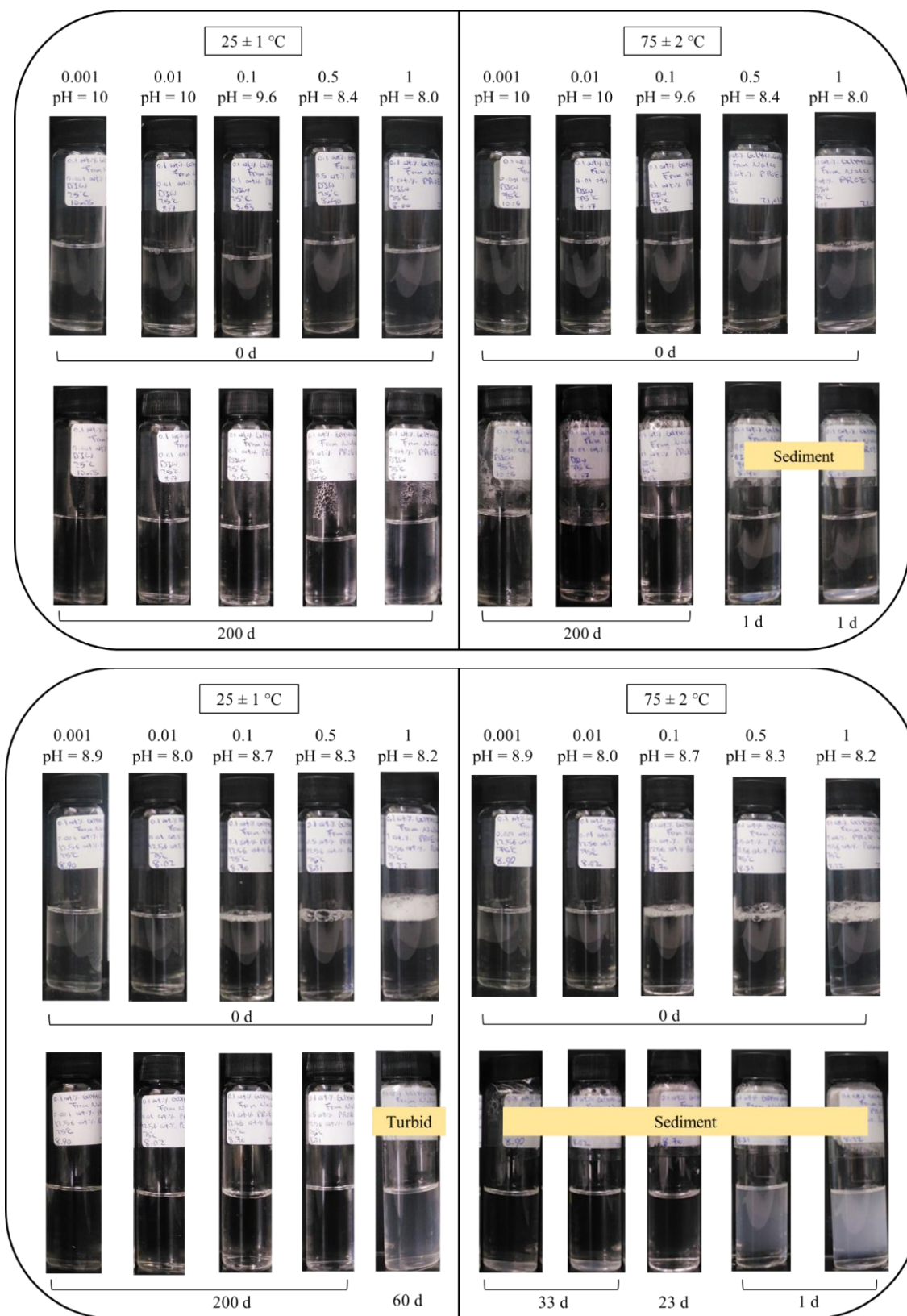
Figure 3.33. Appearance of dispersions containing 0.1 wt.% ES-coated silica in a blend with different concentrations of ZN surfactant in DIW (top) and Permian brine (bottom) at original pH at two temperatures.
