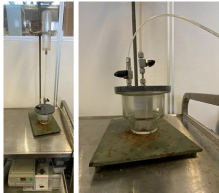
Figure 2.21. Setup used for vacuum saturation of shale cores with heptane.
