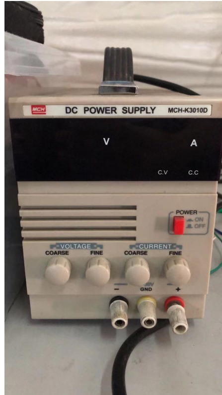
Figure 7.2: Direct current power supply .
