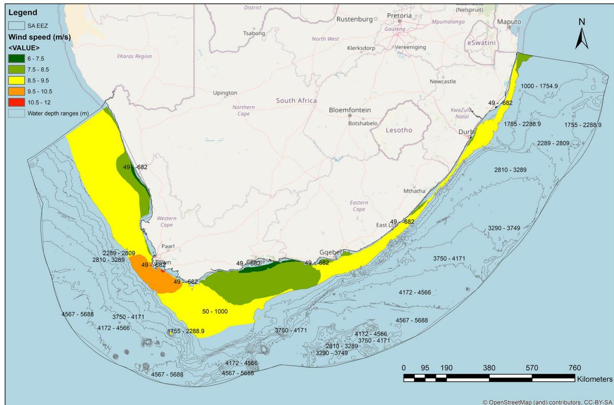
**Fig. 3** Technically feasible zones for FOW development in SA (data sources: GEBCO, 2022; Global Wind Atlas, 2022)
