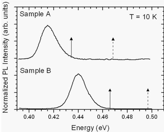
FIG. 2. PL spectra from asymmetric InAs/GaSb SPSLs. Samples A and B have InAs/GaSb layer thicknesses of 1.0/1.7 and 0.9/2.0 nm, respectively. The spectra are offset for clarity. Arrows indicate the calculated energy-gap values: dashed lines for abrupt interfaces and solid lines for graded interfaces.
