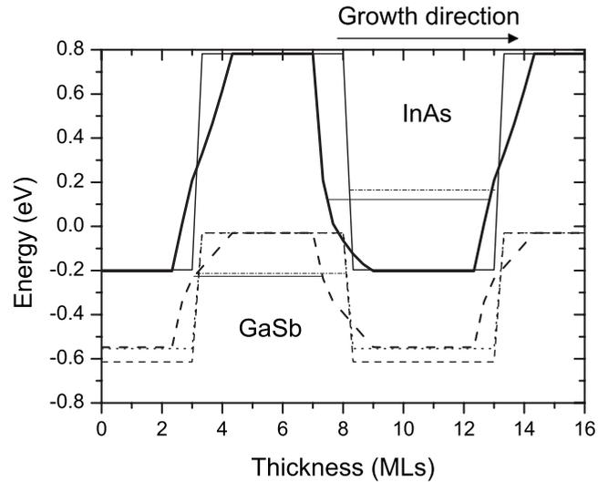
FIG. 4. Band profiles for abrupt and segregated interfaces (fine and bold lines, respectively). Conduction band, light-hole, and heavy-hole valence bands are represented by the solid, dashed and dotted lines, respectively. The ground electron and heavy-hole energy levels are shown for both segregated and abrupt profiles using solid and dash-dotted lines, respectively.
