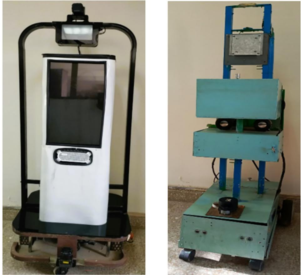
**Fig 3.** The robotic mapping platforms (left) an assistive mobile robot equipped with 2D Hokuyo laser scanners (right) an industrial mobile robot equipped with 2D RPLidar laser scanner.
