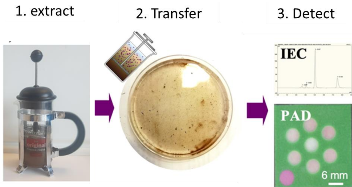
Figure 1.15 The overall workflow which consisted of three steps, cafetière extraction, transfer and PAD detection.
