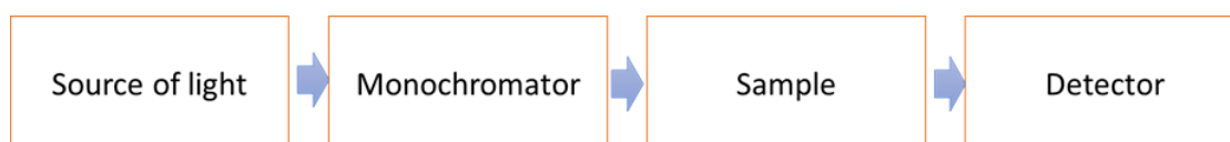
Figure 1.1 Steps for detection of analyte by UV-Vis spectrophotometer.
