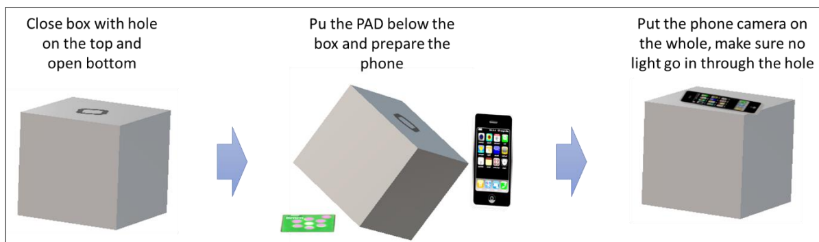
Figure 5.3 Steps for using the box for image capture. The box is closed with hole on the top and open bottom. The PAD is put below the box. The phone camera is attached to the hole of the box and image was then captured of the PAD.
