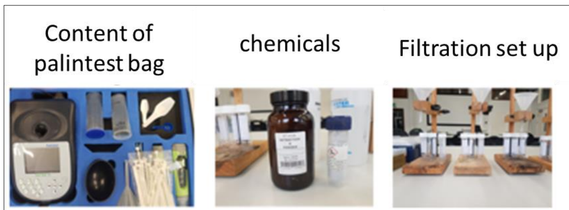
Figure 4.64 Palintest is commercial tests which was used for soil nutrient determination included nitrate. chemicals were bought separately. Filtration was required.
