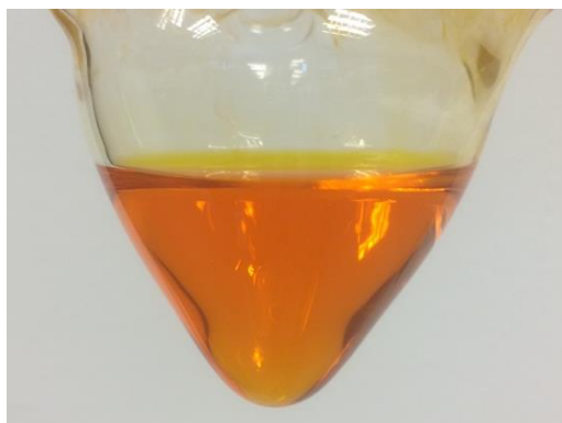
Figure 7.2 - A picture showing the orange coloured solution formed when disodium rhodizonate (4 mM) is dissolved in aqueous KCl (0.1 M) with boric acid (0.1 M).
