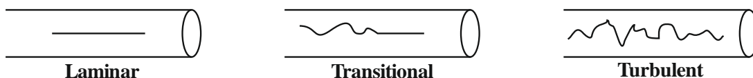
Figure 2.25 - Schematics showing the variations between laminar, transitional and turbulent flow in hydrodynamic systems.
