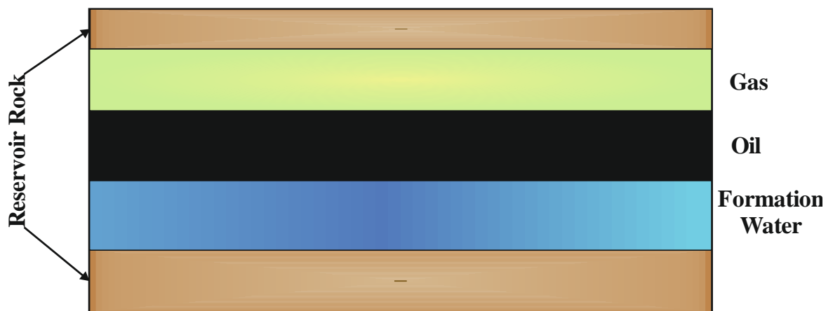
Figure 1.3 - A schematic showing the typical structure of an oil reservoir.
