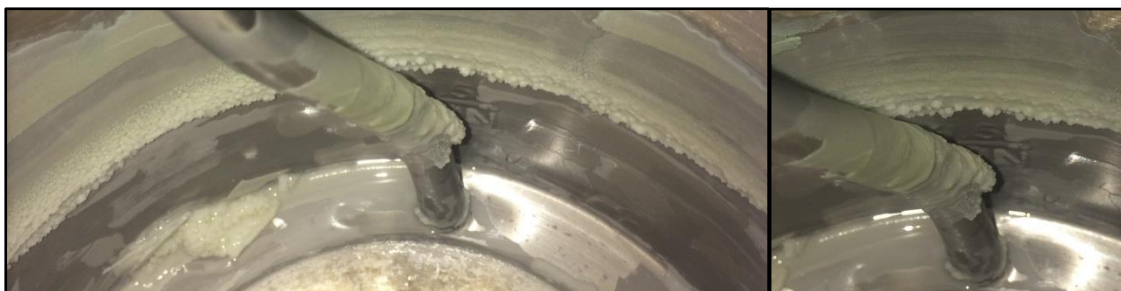
Figure 1.1 - An image showing the build-up of limescale on the inside of a kettle.
