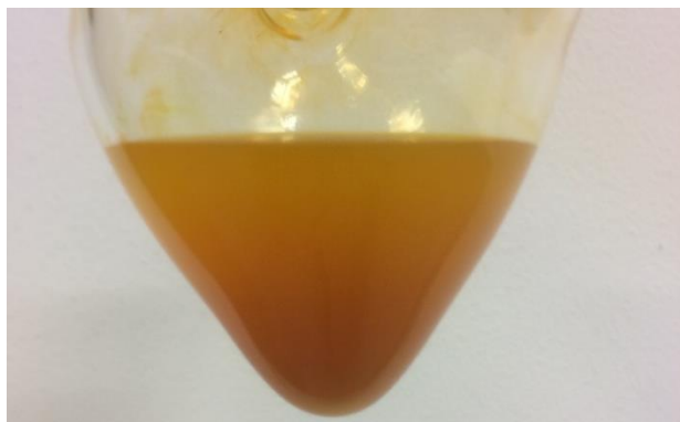
Figure 7.8 - A picture showing the orange coloured solution with dark precipitate formed when disodium rhodizonate (4 mM) is dissolved in aqueous KCl (0.1 M) with boric acid (0.1 M) with \text{Ba}(\text{NO}_3)_2 (4 mM) added to it.
