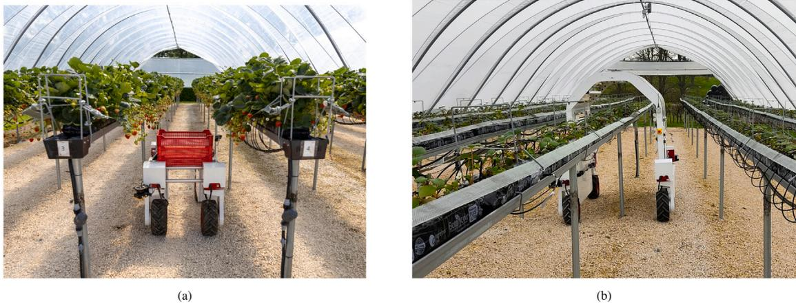
Fig. 1. The Thorvald II configuration used to: (a) perform logistics and picking during fruit harvesting operations; and (b) perform the UV-C treatment and crop monitoring.
