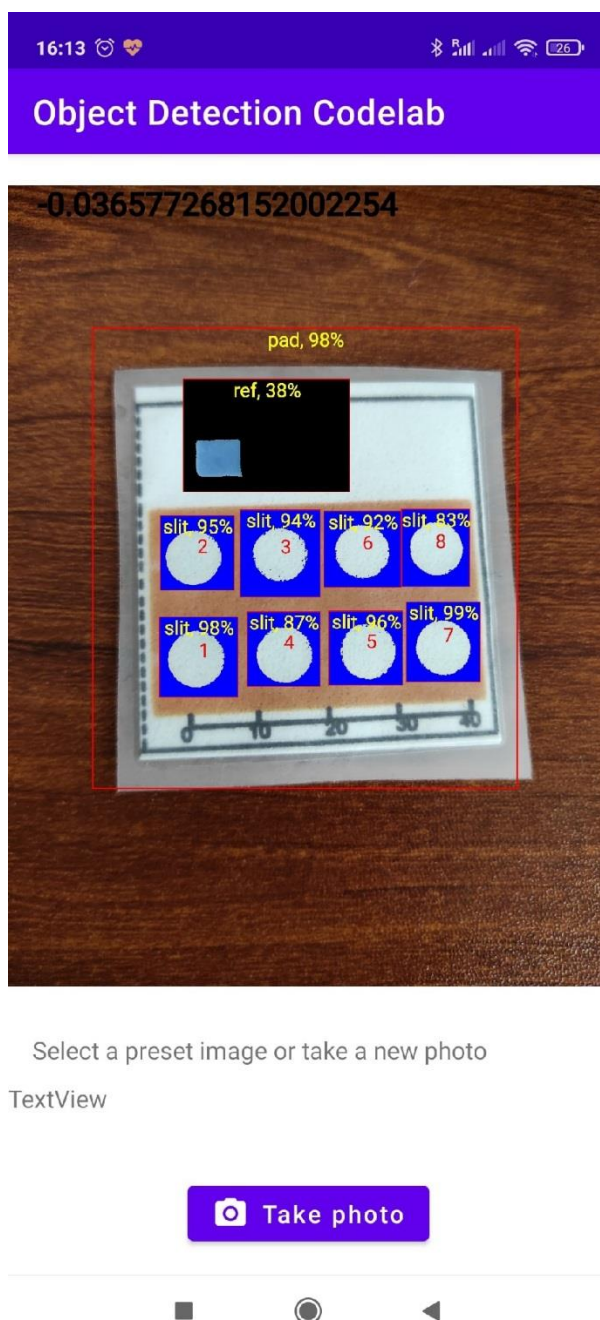
Figure 65. Screenshot of object detection application showing detection result (PAD, reference square and reaction zones).
