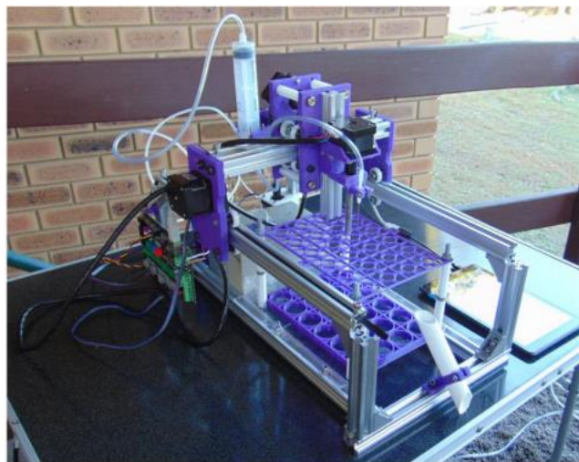
Figure 11. Portable autosampler for discrete surface water samples [51].
