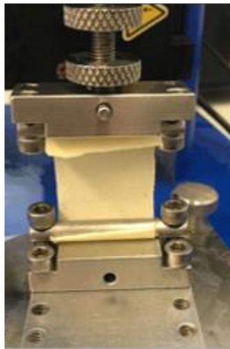
**Figure 7** An illustration of the experimental tensile testing set up used by Griffin et al. (2016). A sample of a synthetic biomaterial can be seen between the clamps.
