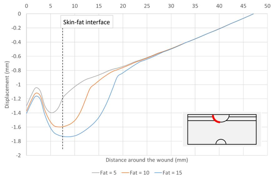
**Figure 42** The distribution of horizontal displacement around the circumference of the wound when the thickness of subcutaneous fatty tissue is varied. The greater the fat thickness, the greater the displacement.
