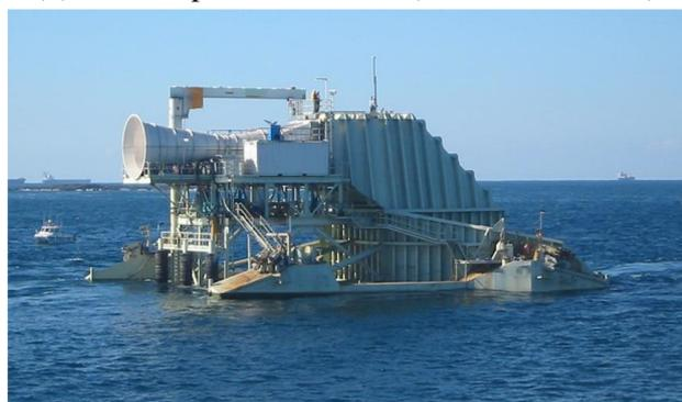
(b) The Oceanlinx WEC device (Delmonte et al., 2014).
