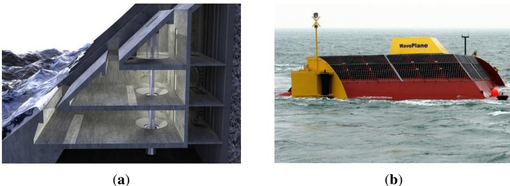
Figure 2.13: The structure of overtopping WECs, (a) SSG WEC (Vicinanza et al., 2012), (b) Waveplane WEC (WavePlane, 2008).
