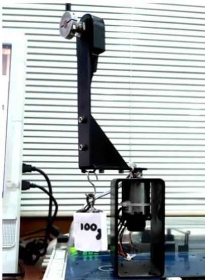
FIGURE 13. Pendulum setup with 0.10 kg mass attached to arm [34]
