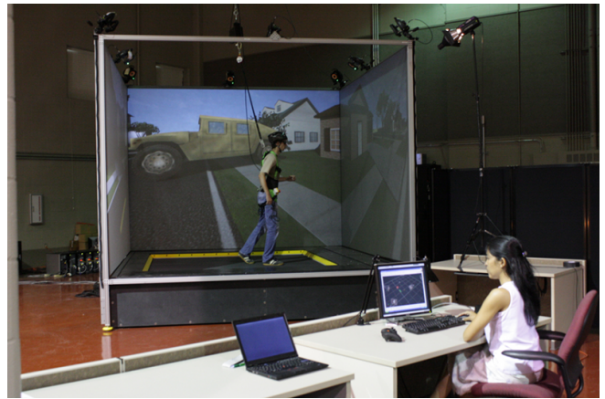
Figure 2: Omni-directional treadmill system in operation. The walkable area of the omni-directional treadmill can be seen surrounded by yellow markings.
