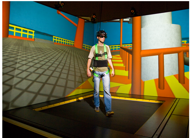
Figure 1: An immersive simulator running in our surround-screen display system with the omni-directional treadmill.
