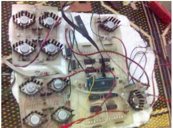
Fig. 5 Complete electronic circuitry of the PR robot manipulator
