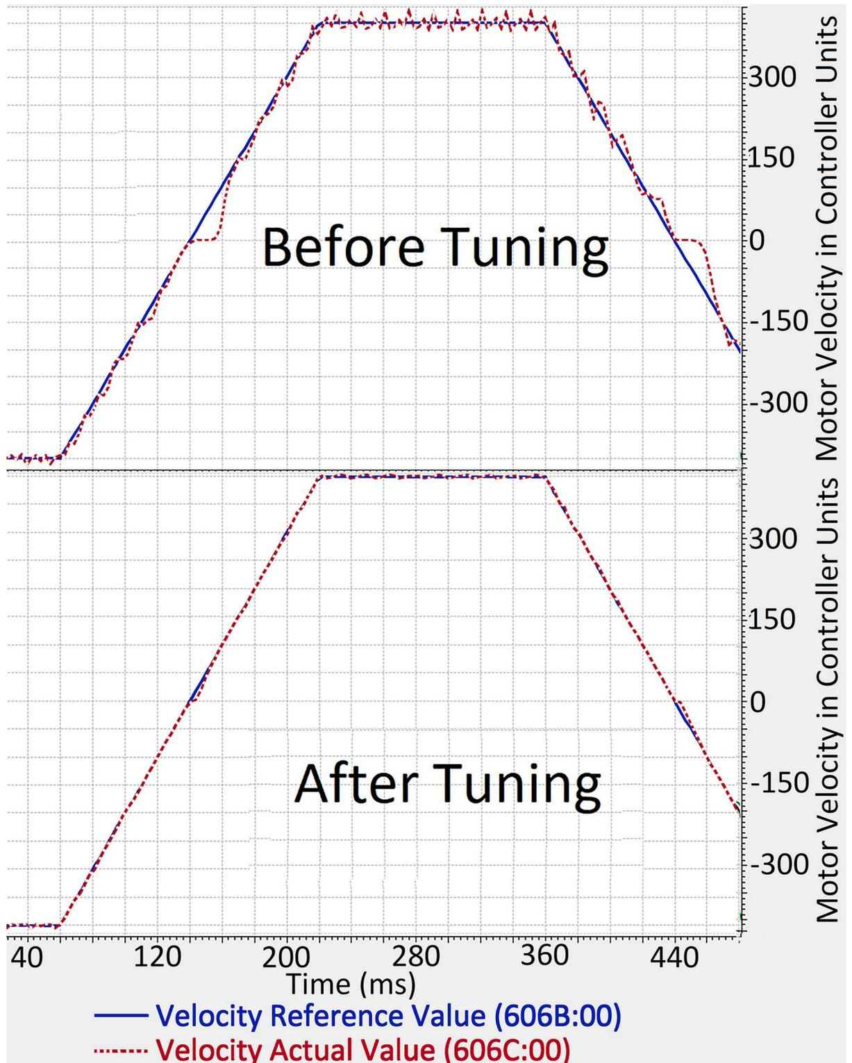
**Fig 21.** Before and After tuning response of position (left) and Velocity (right) of one of the joints. The x-axis shows time in milliseconds, whereas y-axis shows the position and velocity in motor controller units.
