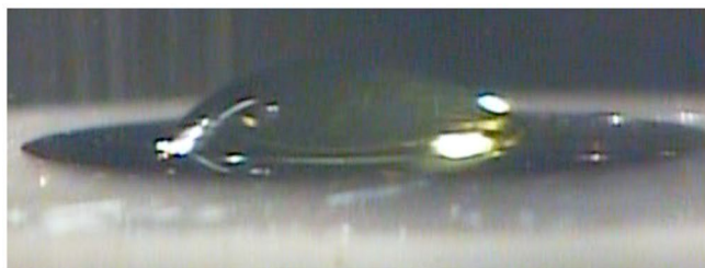
Fig. 8 Photograph (left) of a droplet of nitrobenzene containing TPPD (9.7 mM) and {}^n\text{Bu}_4\text{NClO}_4 (0.1 M) immobilised on the surface of a glassy carbon electrode and surrounded by a 0.1 M aqueous KCl solution. The electrode potential is 0.0 V vs. SCE. The plot (right) is of the co-ordinates of the liquid/liquid interface (red points) extracted
