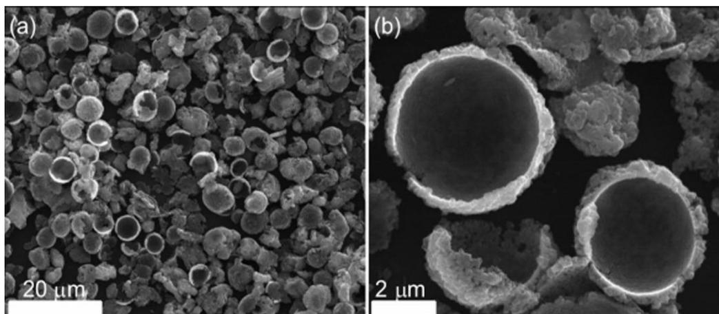
**Figure 2.** SEM images of the silica shell fragments obtained by templating yeast cells.
