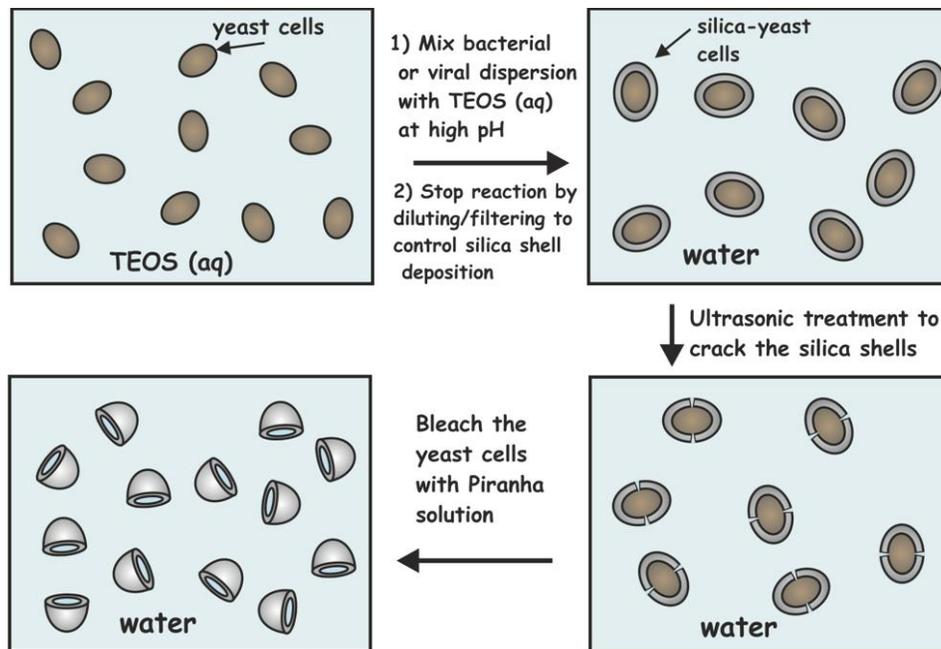
**Figure 1.** Fabrication scheme of the novel nanoantibiotic particles. The nanoantibiotic particles were fabricated via silica deposition onto yeast cells templates which was followed by the silica shell fragmentation and cell removal via a bleaching process. These inorganic templates of the yeast cells surface were then used to test the shape and size recognition in a dispersion of yeast cells as well as a mixture of yeast and other bacterial cells.
