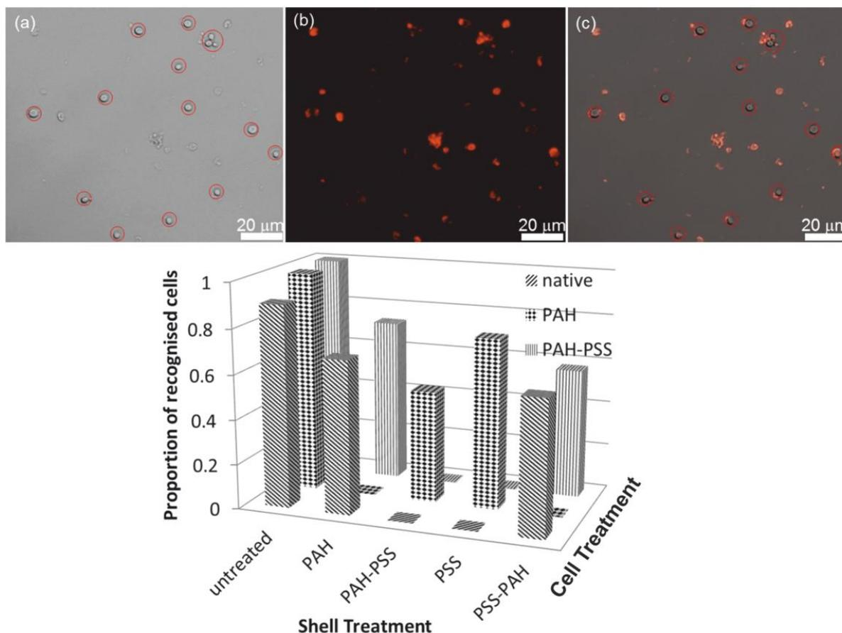
**Figure 4.** A cell recognition experiment which involved untreated yeast cells and untreated silica shell fragments leading to a match of the silica shell fragments and their cell targets. The bright field image (a) and the fluorescence image (b) were overlaid to produce the image (c). The diagram summarizes the findings from the nanoantibiotic-yeast cell recognition experiments.
