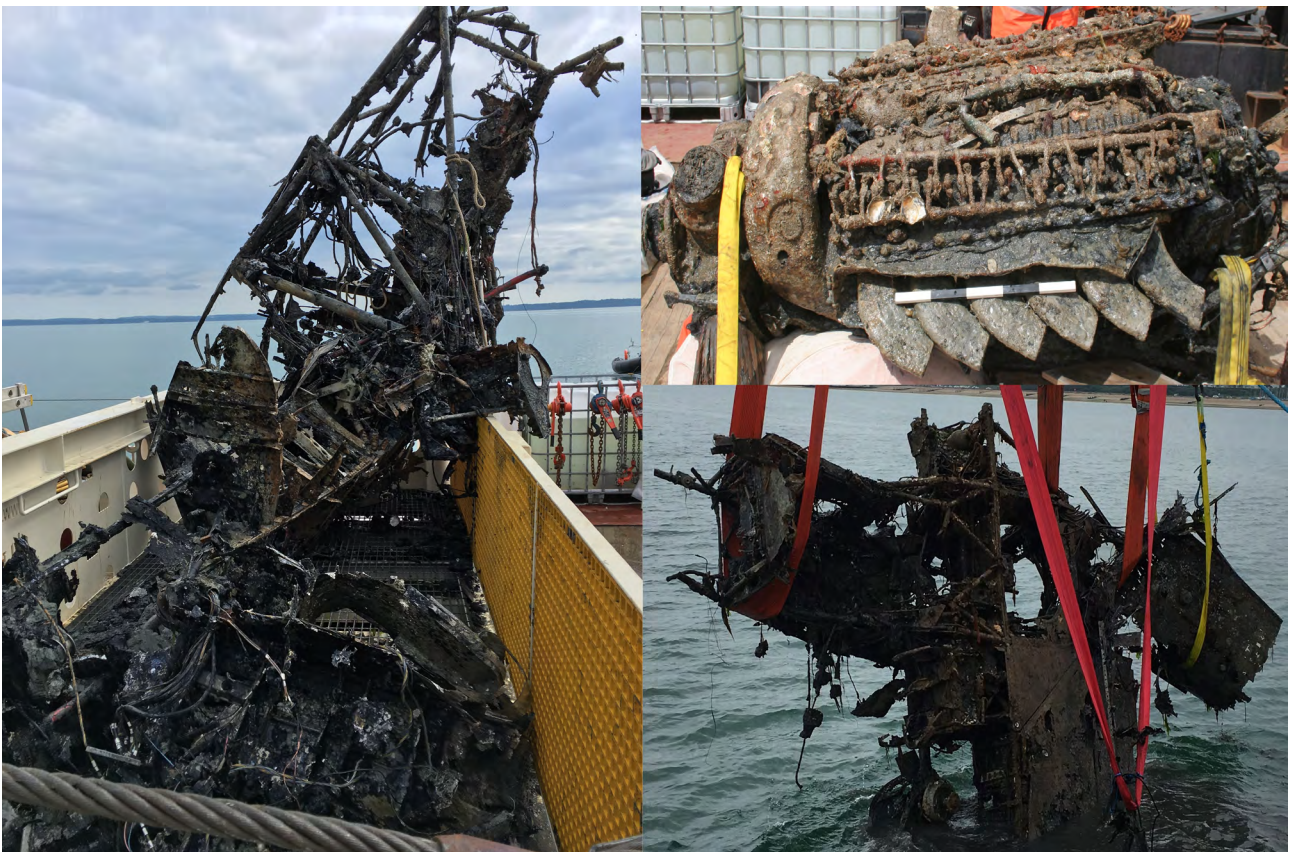
Figure 16.6. (Left) Pilot's cockpit, Observer's cockpit, and wing stubs following recovery with subsea basket. (Right, top) Rolls Royce Merlin 32 engine following separation from airframe and recovery. (Right, bottom) Aircraft during initial lift attempt. All images copyright Wessex Archaeology.
