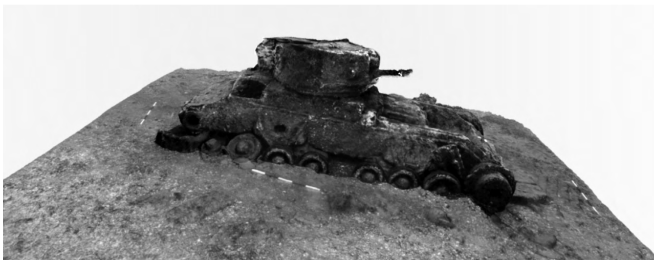
Figure 18.2. Underwater Photogrammetry of the complete (before the damage that occurred during 2022) ‘Tank 1’ (Valentine MK-IX DD) at the bottom of Studland Bay (3D model of 3.3 million vertices in 6.6 million triangles). Without a fixed survey grid on the tanks, the ‘rapid fire technique’ developed by Daniel Pascoe (Pascoe Archaeology Services) and Bournemouth University was used, employing a goPro6 camera with a 105 degree fisheye lens. Four one-meter scale bars were placed around the site, and then with the goPro’s time-lapse function, photos were automatically taken every second, with the diver slowly swimming over the site. The resulting photos were colour corrected using Adobe Photoshop and loaded into Agisoft Metashape where the images were further processed to mask out any undesirable features, such as the water column and fish, and to calibrate the lens to compensate for the wide angle which can cause issues with alignment. After processing and filtering with Metashape, the original photos were then used to create the texture-map. Finally, the model was scaled using the bars placed around the site during image acquisition before it was exported as a 3D object. Image created by the Exercise Smash Development Team.
