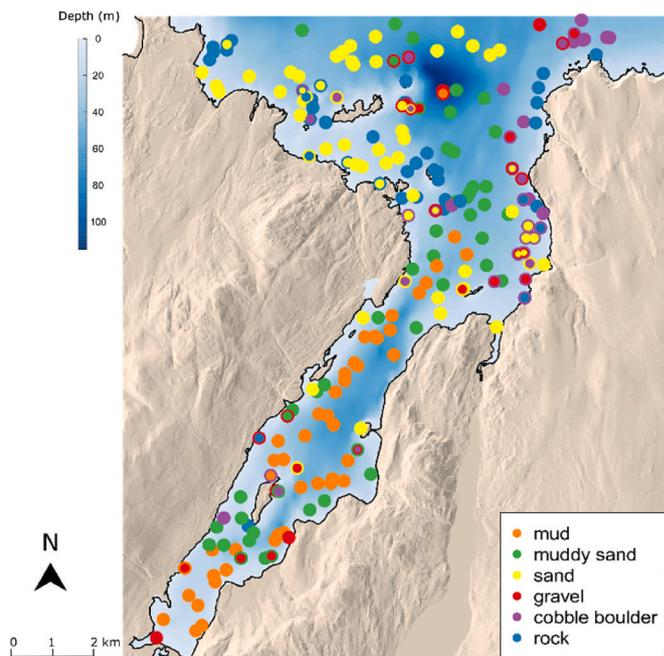
Fig. 3. Substratum category observed at each sample site from video collected in 2021. Coloured discs correspond to substrata classification(s) visible in the field of view of one stereo video camera. Where multiple substratum categories exist at one location up to three sizes of circles are used to indicate all substratum categories visible.
