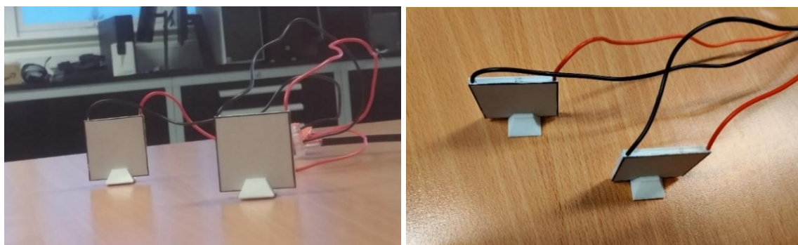
Figure 35 - TEC modules arrangement shown from front view (left) and top view (right)
