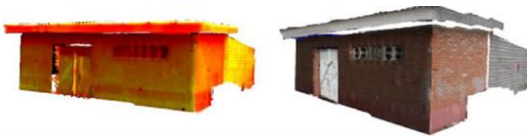
Figure 16 - Thermal 3D Model (left) and its corresponding RGB 3D Model (right) [124]
