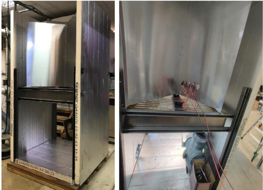
Figure 84 – Four-quadrant section (left) and the cooling unit underneath (right)
