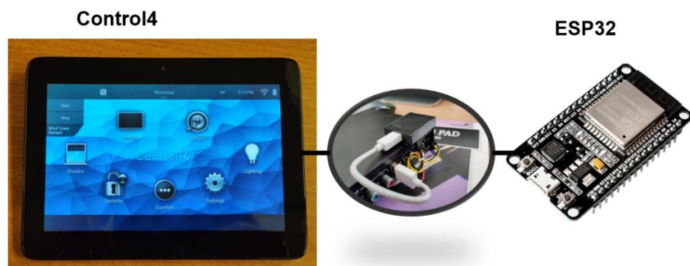
Figure 55 – ESP32 Microcontroller and its integration with Control4 UI
