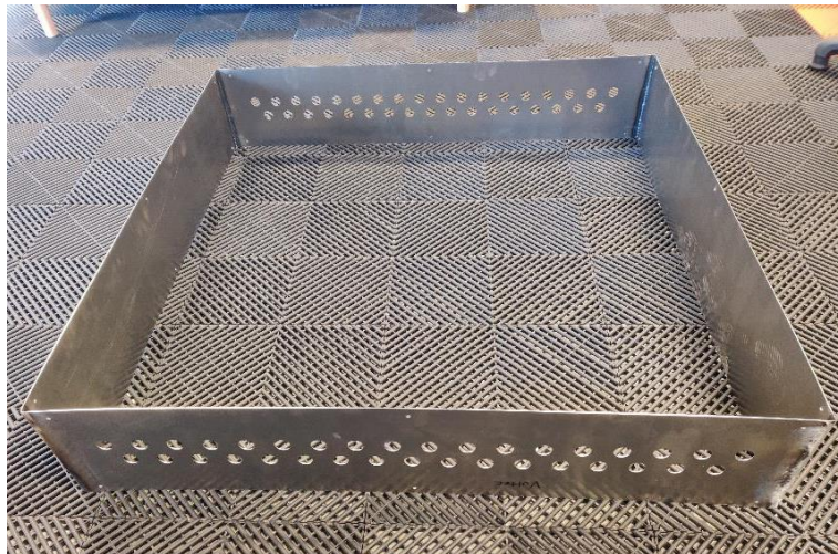
Figure 81 – Aluminium frame for full-scale prototype
