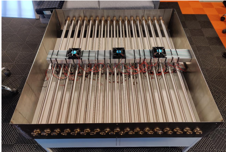
Figure 82 – Fully assembled prototype of the TEC cooling unit for experiment 5
