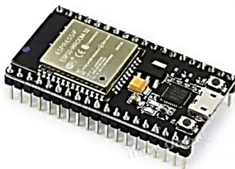
Figure B3 – ESP32 Wroom-32 device and specifications [221]
