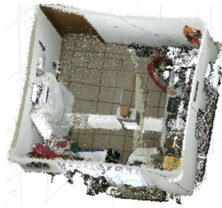
Figure 13 – Point cloud fusion via four Kinect sensors [116]
