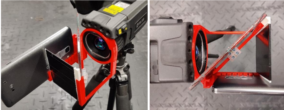
Figure 33 – Image fusion module with cameras mounted shown from two angles
