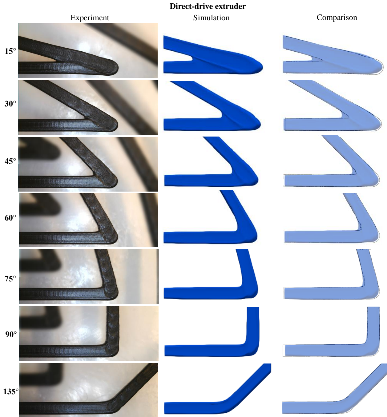
Figure 4: Microscopic images of corners of different angles using Direct extruder (left column), simulated results (middle column), and comparison between simulations and experiments (right column).
