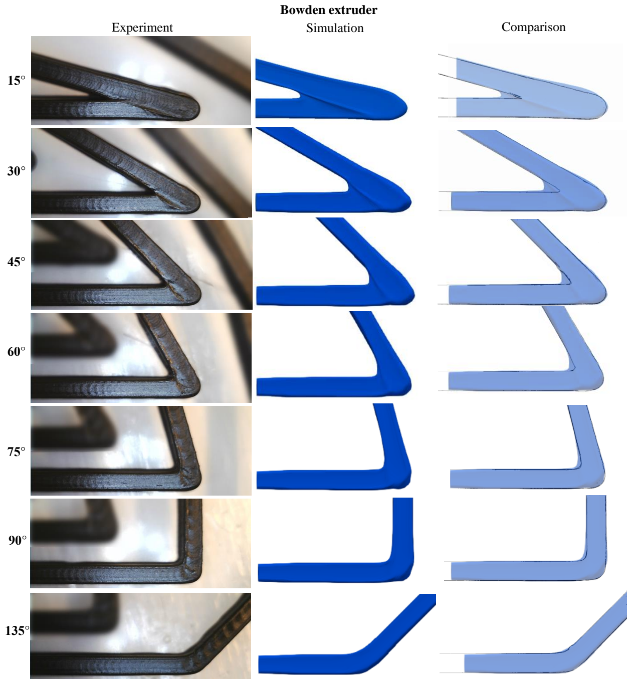
Figure 3: Microscopic images of corners of different angles using Bowden extruder (left column), simulated results (middle column), and comparison between simulations and experiments (right column).
