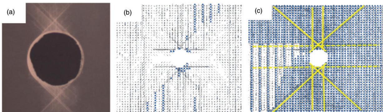
**Figure 16.** Damage zones associated with  $[45^\circ/0^\circ/-45^\circ/90^\circ]_{2s}$  IM7/8552 CFRP composite specimens: (a) X-Ray experimental result,<sup>41</sup> (b) damage zone represented by cracks at strain of 0.58%, (c) damage zone represented by cracks at strain of 0.73%.
