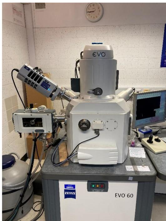
**Figure 14: Zeiss Evo 60 SEM with an Oxford instruments X-Max 80**
