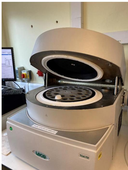
**Figure 11: Figure 10: LECO TGA 701 thermogravimetric analyser for multiple, large samples under parallel conditions.**
