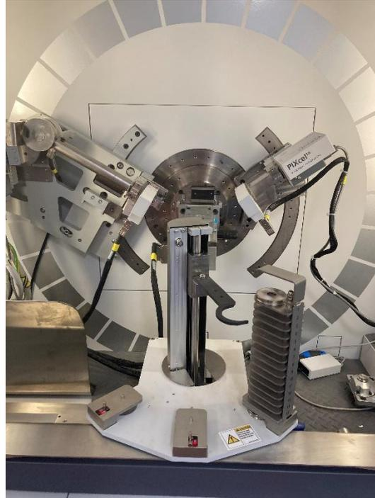
**Figure 17: PANalytical Empyrean series 2 diffractometer.**
