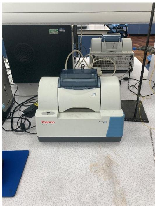
**Figure 10: Thermo Scientific Nicolet iS5 without the PIKE MIRacle single reflection horizontal ATR accessory.**
