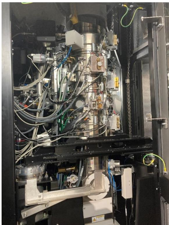
**Figure 15: FEI Titan3 Themis 300 Transmission Electron Microscope
