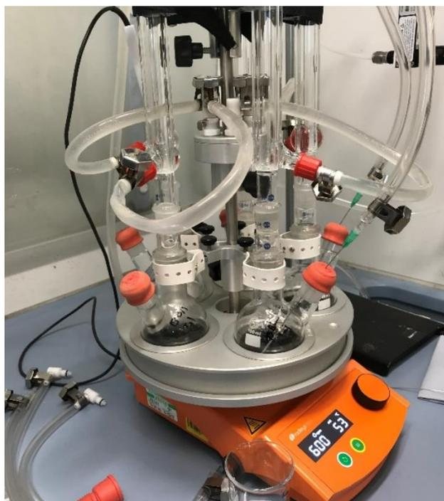
**Figure 8: Radleys Starfish parallel reactor platform operating the hydrogenation of four reactions simultaneously.**
