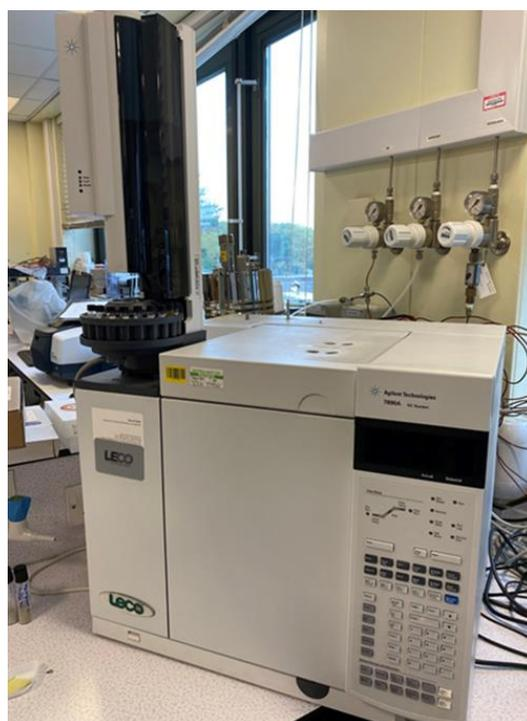
**Figure 9: LECO-Agilent Technologies 7890A Gas Chromatograph with flame ionisation detector.**
