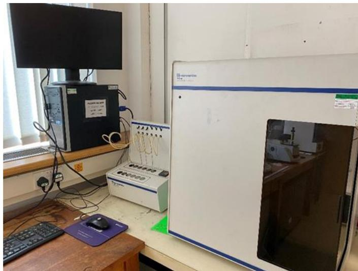
**Figure 16: Micromeritics TriStar Surface Area and Porosity Analyzer with degassing station.**
