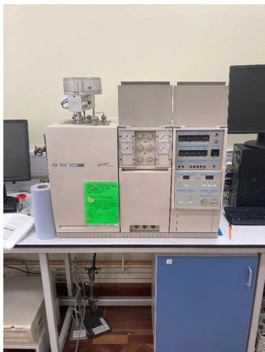
**Figure 13: Fisons Instruments EA 1108 CHNS elemental analyzer**
