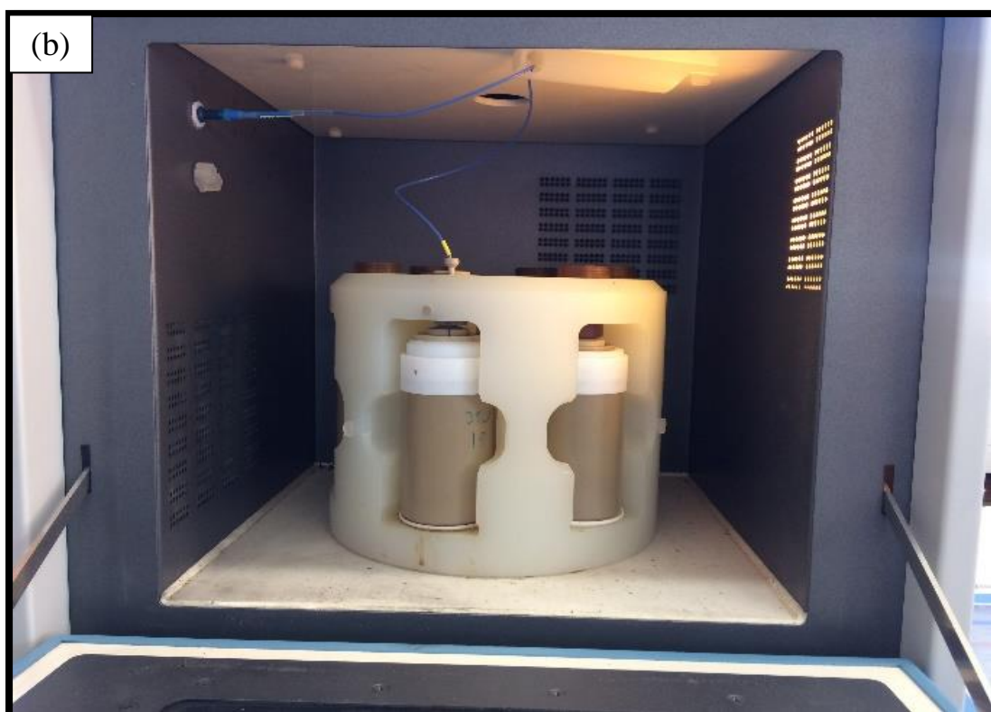
Figure 2-3. Ethos EX microwave and the PTFE rotary vessel reactors system: (a) Schematic and (b) picture.
