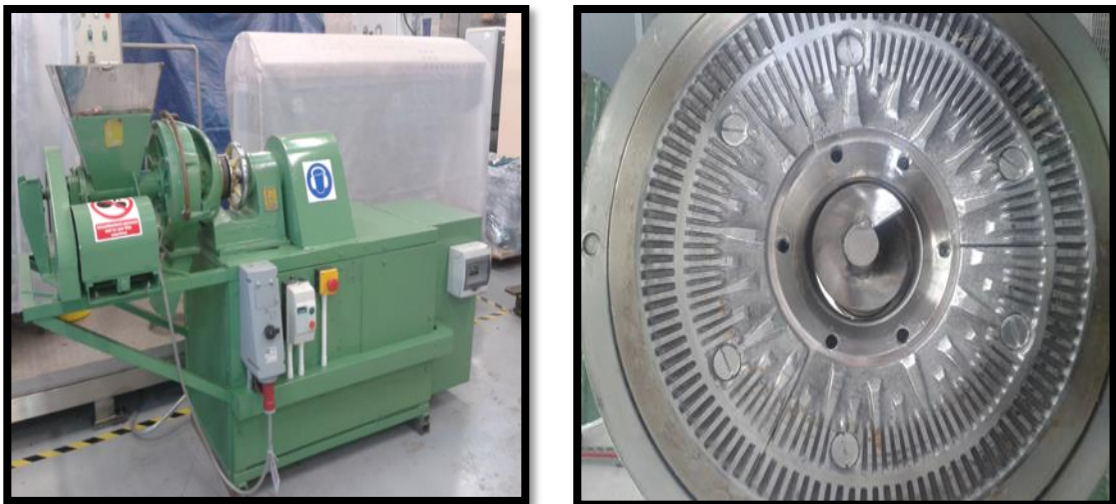
Figure 2-4. Atmospheric disc refining equipment and the refiner plate (Bangor University).
