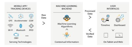
Fig. 12.1 Future mobility sensing (FMS) platform architecture
