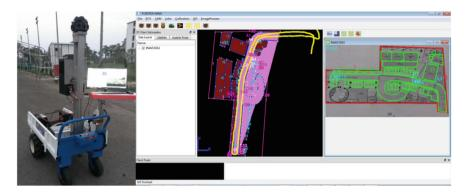
Fig. 25.10 Indoor mobile mapping technology
