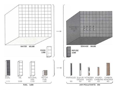
Fig. 7.2 Wolman's 1965 urban metabolism of a hypothetical American city of one million people, focusing on water, food, and fuel as inputs and on sewage, solid waste, and air pollutants as outputs
