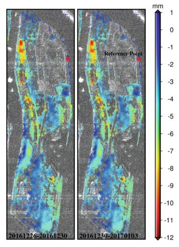
Fig. 21.8 Deformation map over a man-made island in Macau from three COSMO-SkyMed images and DInS AR processing
