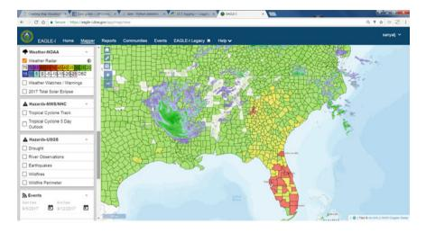
**Fig. 18.6** Eagle-I<sup>TM</sup> displaying locations of over 7 million customers who lost electricity as an aftermath of Hurricane Irma in the southeastern USA during September 2017
