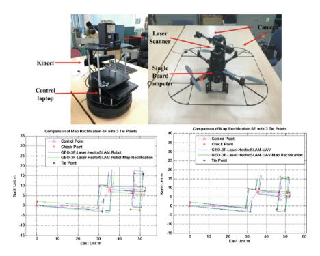
Fig. 25.16 An example of unmanned mobile mapping technology
