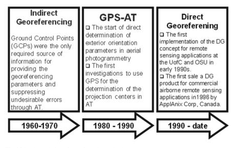
Fig. 25.1 The evolution of georeferencing technology
