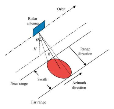
**Fig. 21.1** Typical SAR imaging geometry. The antenna receives the backscattered signal from the illuminated area. The moving direction of the satellite is called the azimuth direction of the image, while the direction of radar illumination is referred to as the range direction of the image. *H* and *R* are the height of the satellite and the slant range between the satellite and a ground resolution cell, respectively.  $\theta$  represents the look angle
