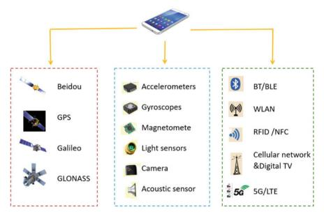
Fig. 26.1 Multiple sensors embedded in the smartphone
