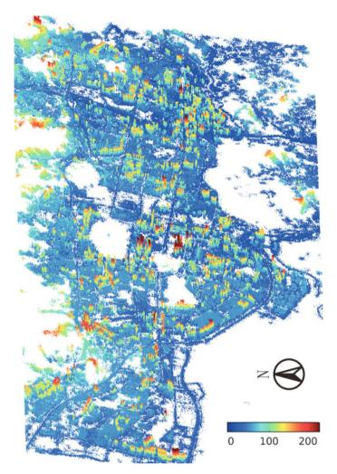
Fig. 21.5 Surface elevation model of part of Shenzhen from 79 TerraSAR-X images and MTInSAR processing
