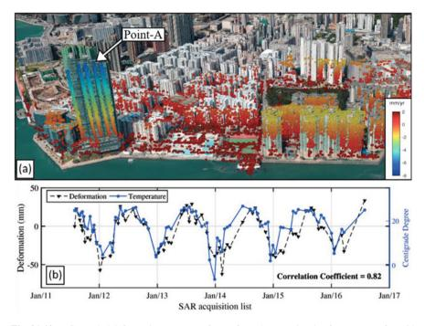
**Fig. 21.10** a Geocoded deformation rate map of part of Kowloon Peninsula of Hong Kong from 80 COSMO-SkyMed images and MTInSAR processing. The map is superimposed on a Google Earth image (© 2019 Google). **b** Deformation time series and temperature variations of Point-A
