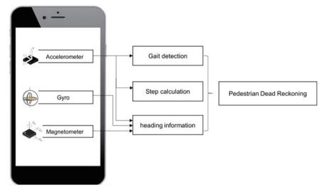
Fig. 26.2 PDR system block diagram
