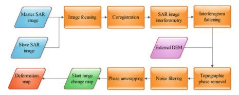
Fig. 21.4 Workflow of DInSAR processing for extracting a deformation map
