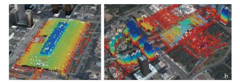
**Fig. 21.6** Geocoded height maps of buildings over Shenzhen. **a** Shenzhen Convention & Exhibition Center, **b** Shenzhen Citizen Center. The maps are superimposed on a Google Earth image (© 2019 Google)
