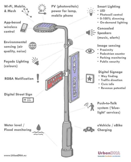
Fig. 38.6 Sensors on the humble lamp post, UrbanDNA (2018).
