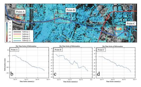
**Fig. 21.9** a Deformation rate map along a metro line in Shenzhen from 50 TerraSAR-X images and MTInSAR processing; **b** Deformation time series of Point-A; **c** Deformation time series of Point-B; **d** Deformation time series of Point-C
