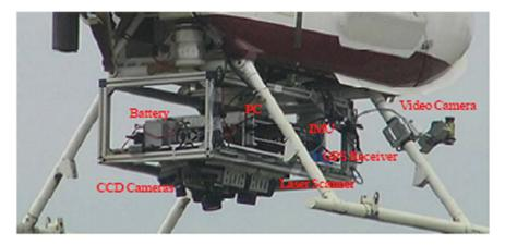
**Fig. 25.5** An example of a DG-ready UAV helicopter-based photogrammetric platform. Adopted from Nagai et al. (2008, p. 1217)
