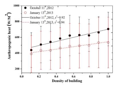
Fig. 20.12 Relationship between anthropogenic heat and building density
