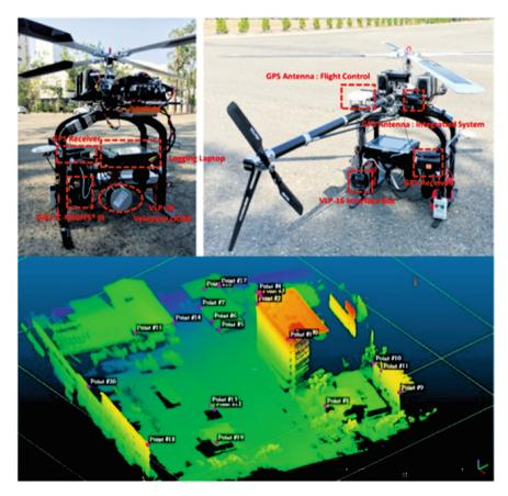
Fig. 25.6 An unmanned helicopter-based LiDAR mapping system
