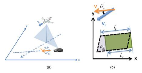
Fig. 22.3 Moving objects undergo the scanning of airborne LiDAR. Copyright © 2010 IEEE, reproduced by permission
