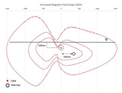
**Fig. 24.1** a Experimental setup in HK PolyU's underground utility survey lab: *X*: horizontal separation (350, 550, 750, or 950 mm) *Y*: vertical position (150, 300, or 450 mm); **b** estimated magnetic field shape for a cable at 150 mm depth and separated horizontally from the pipe by 350 mm
