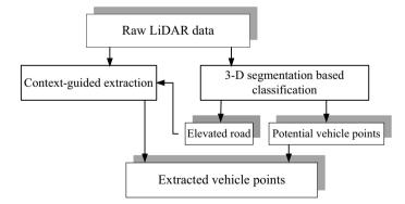
Fig. 22.6 Workflow for vehicle extraction
