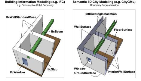
Fig. 34.7 Geometry modeling paradigms predominantly applied in BIM and semantic 3D city modeling (Nagel et al. 2009)
