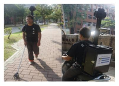
Fig. 25.7 Example of portable mobile mapping systems
