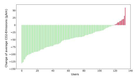
Fig. 6.2 Comparison of SBB Green Class 1 users' average  $CO_2$  emissions during a six-week preproject tracking phase and their emissions after they got access to the new mobility tools (public transport pass, e-car, etc.). Most participants (indicated in green) were able to reduce their  $CO_2$ emissions significantly and only few participants (indicated in red) increased their average  $CO_2$ emissions compared to before the project
