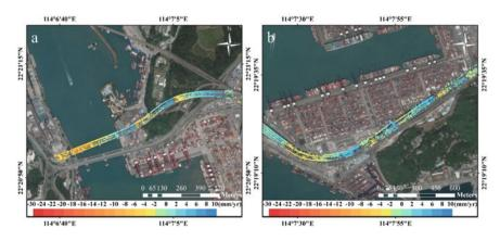
Fig. 21.11 Examples of road viaduct deformation in Hong Kong from 29 TerraSAR-X images and MTInSAR processing. **a** Tsing Kwai highway, **b** Tsing Sha highway
