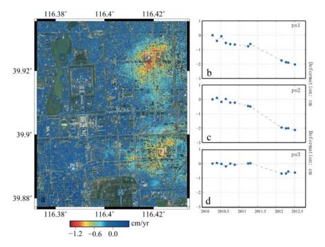
Fig. 21.7 a Deformation rate map over Beijing from 12 TerraSAR-X images and MTInSAR processing; b Deformation time series of ps1; c Deformation time series of ps2; d Deformation time series of ps3
