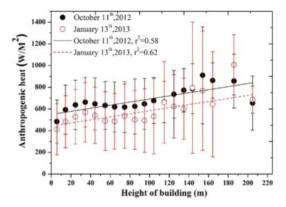
Fig. 20.11 Relationship between anthropogenic heat and building height
