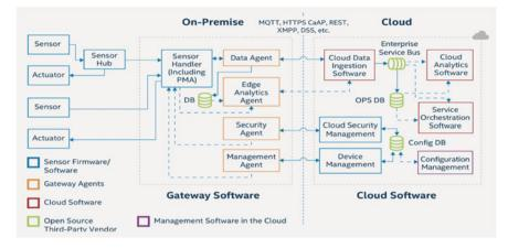
Fig. 38.3 Intel IoT reference architecture (Intel 2018).
