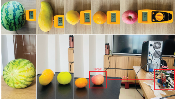
Fig. 17: Experimental setup for mmFruit and ground truth moisture estimation using commercial off-the-shelf (COTS) devices.
