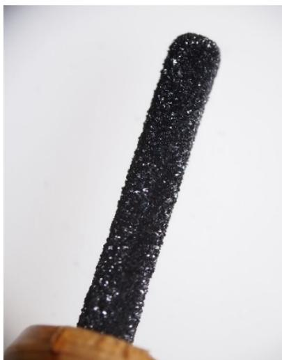
**Figure 2.** Photograph of a platinum rod electrode covered with crystals of compound **2b**.
