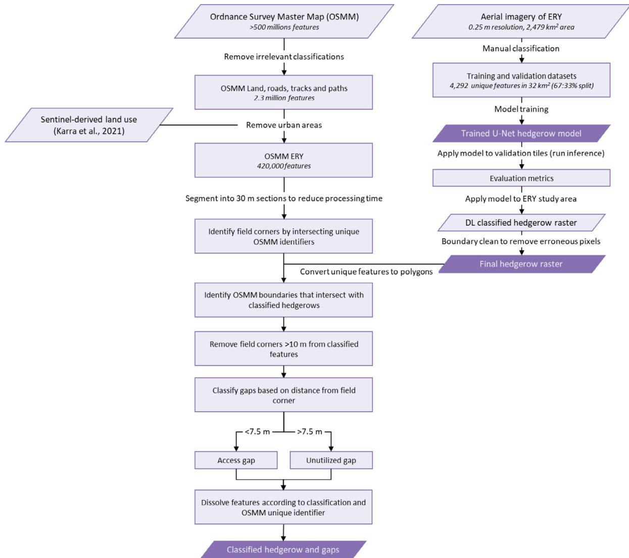
**Figure 2.** Process diagram for generating the DL model and detailing the extraction of hedgerow gaps from the OSMM dataset.
