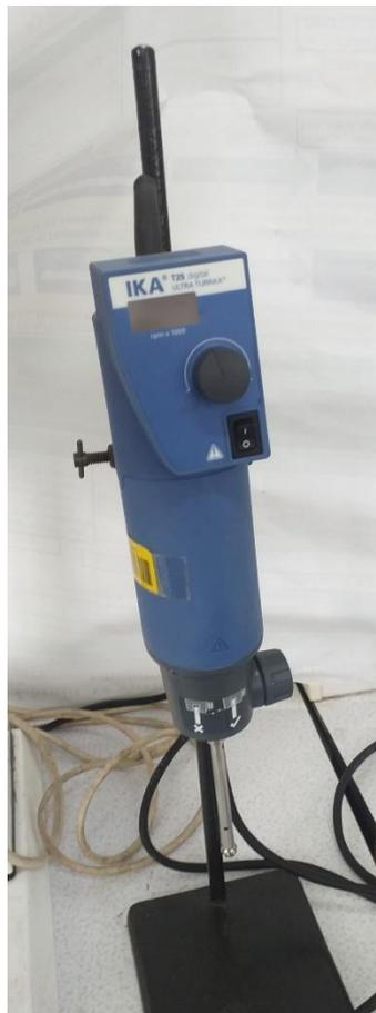
**Figure 2.2** Photo of Ultra-Turrax T-25 homogenizer.
