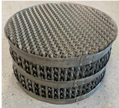
Figure 2: - BX Packing used in absorption column
