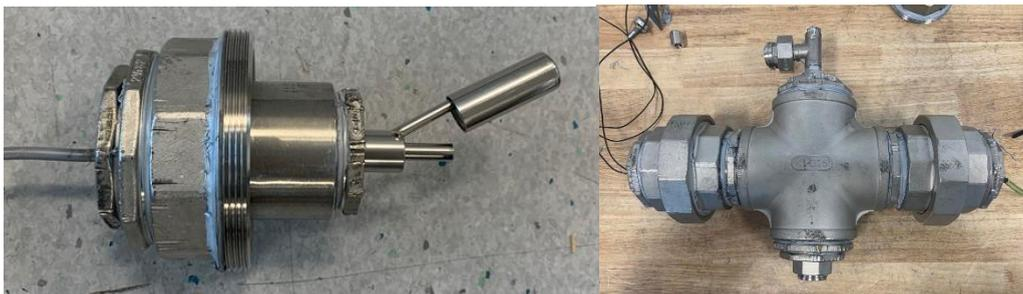
Figure 3: - Liquid release system internals (left), and external (right)
