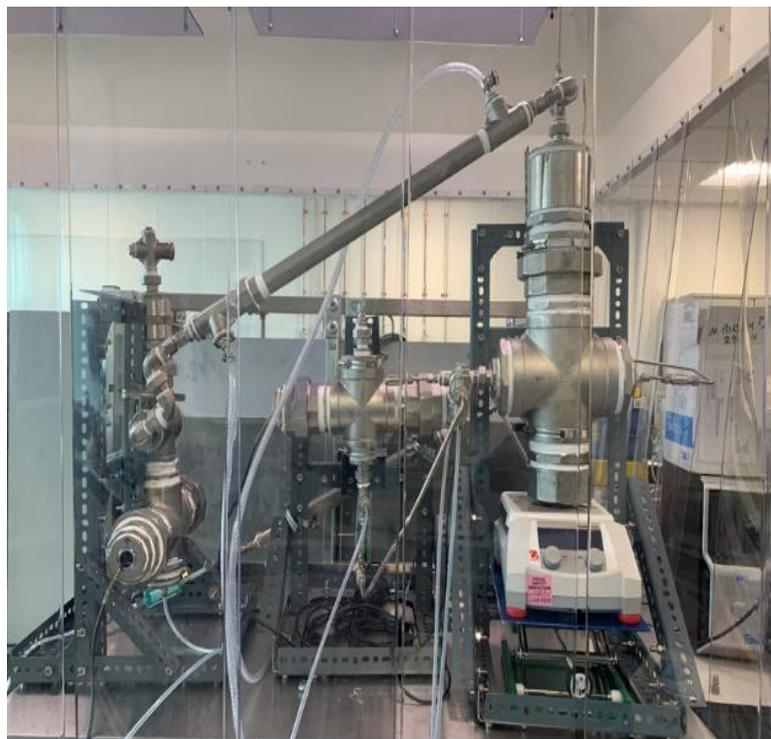
Figure 2. Prototype First Stage Continuous Reclaimer (Standalone, without heating tape)
