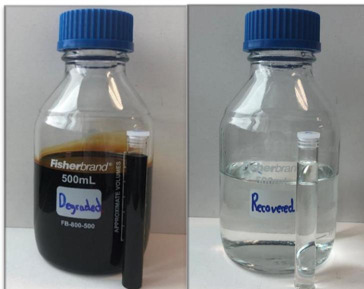
Figure 6. Visual representation of degraded end of life industrial MEA solvent before (left) and after (right) reclaiming. \*Volumes of reclaimed solvent not to scale
