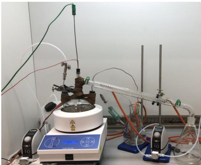
Figure 3. Second Stage Batch Glassware Reclaimer
